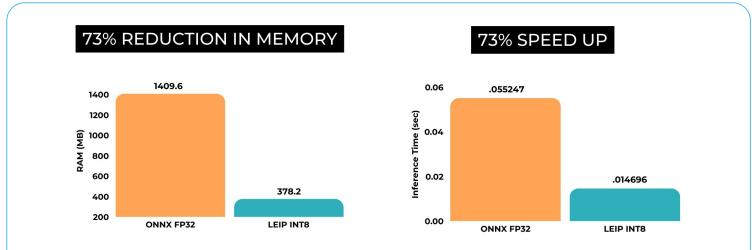
LEIP enables a reduction in RAM usage and interference time. The result is that hardware can be used to process more data quickly. This plot compares EfficientAD on an NVIDIA® RTX™ 5000 Ada Generation GPU.
